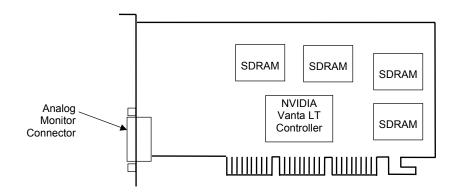
Figure D-1. Compaq/NVIDIA Vanta LT AGP Graphics Card (P/N 192174-002) Layout
